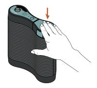
Gently press down to lock the battery in place.
