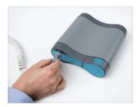
Insert the cable from the connection box to the connection cable socket on the device. Note:
