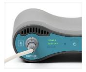
Battery power self-test is complete and the device is turned on when: the red "Error" light turns off and BOTH the "Power" and the "Battery" lights are green.
