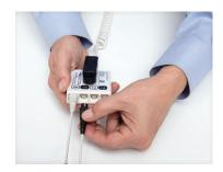
Firmly insert the black and white array wire ends into the corresponding black and white sockets on the connection box
