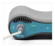
Plug-in power self-test is complete and the device is turned on when: the red "Error" light turns off and ONLY the "Power" light is green.
